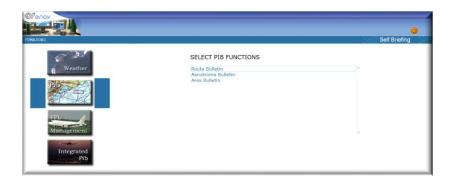
The PIB menu consists of three functions, described below, for NOTAM acquisition in the most appropriate way to your needs.
