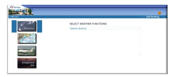
The Weather menu has only one submenu, Weather Briefing, to access meteorological messages, automatically associated to the relevant weather charts useful for flight planning.
