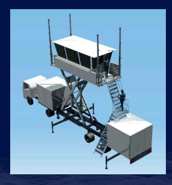
of wind up to 50 kilometers or up to 120 kilometers per hour depending on whether it has no supports or is anchored to the ground.
