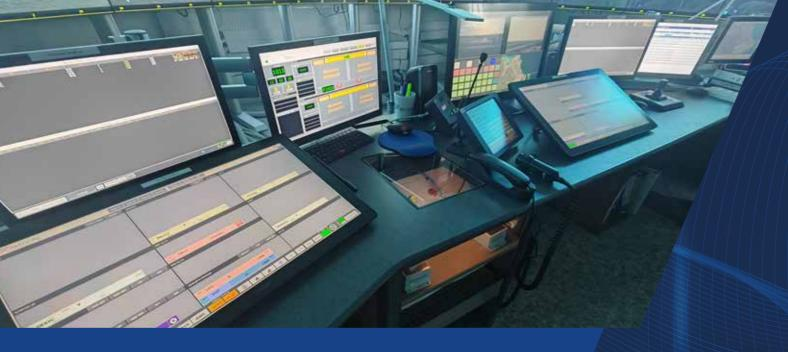
The introduction of remote digital towers represents an epoch-making revolution in the way airport traffic service is provided. The physical control tower is replaced by a digital operations room from which air traffic controllers can operate through the use of cameras and high-definition image monitors. The digital configuration improves the controller's situational awareness, thus offering operational and safety advantages.
