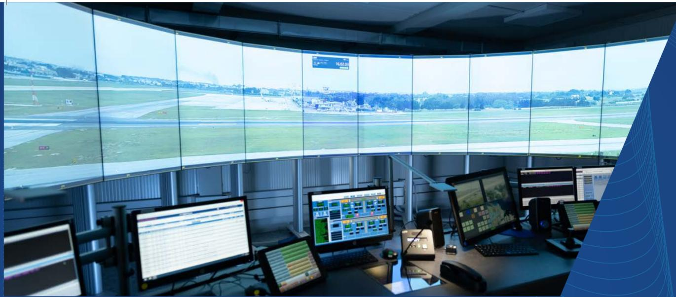
The introduction of remote digital towers will revolutionise the management of airport air traffic services. The physical control tower is replaced by a digital operations room from which air traffic controllers can operate through the use of cameras and high-definition image monitors. The digital configuration improves the controller's situational awareness, thus offering operational and safety advantages.
